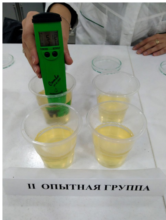
Fig. 2 The process of determining the total acidity level of hone
